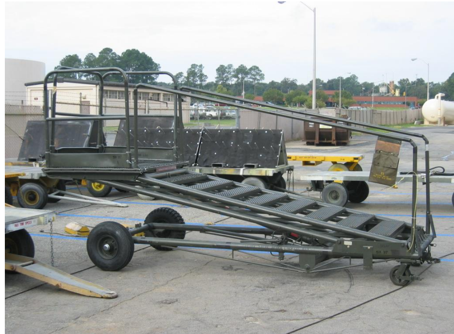
B1 Maintenance Stand
