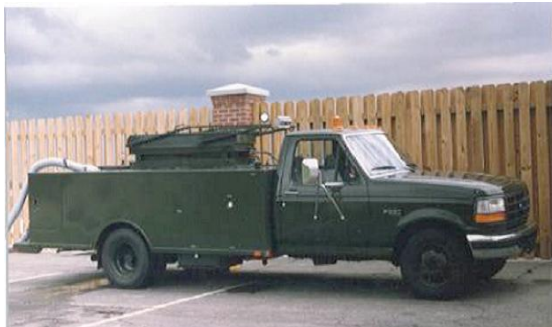
LAVATORY SERVICE TRUCK
